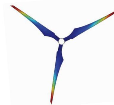
**Activity 2:** Development of models using CFD for wind loading analysis on solar arrays and wind turbines. Field data will be used as validation. Open-source models will be developed for use by practitioners. Figures: wake generated by a turbine rotor (left) and wind loading simulation on non-rotating rotor (right).
