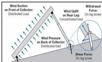
**Activity 2:** Detailed studies of real wind loads on wind turbines and solar arrays will be carried out at the Eolos field station. Data will be used for validating numerical models and developing guidance for engineering design. Figures: Eolos turbine taken from met tower (Left) and simple loading on a solar array (right).
