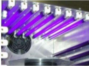
Expose contaminants to UV light, measure how fast they are broken down, generate products for toxicity testing
