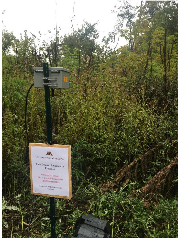
Figure 10. A rotation impaction sampler deployed in Minnieska, Minnesota.
