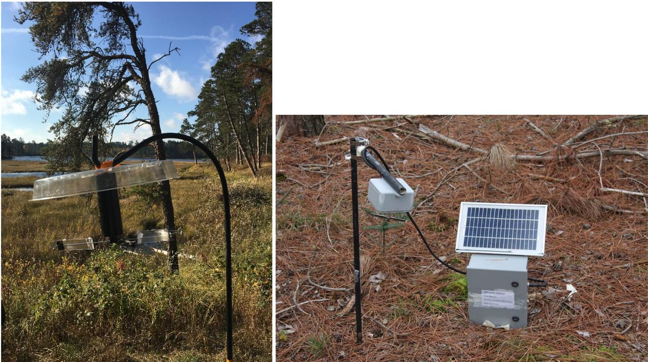
Figure 9. Spore sampler in Itasca State Park (left). A new spore sampler being tested contain two small rods that are programmed to spin at specific time intervals and collect airborne spores. This sampler (right) appears to be more sensitive and efficient at collecting the very small spores produced by *Heterobasidion*.
