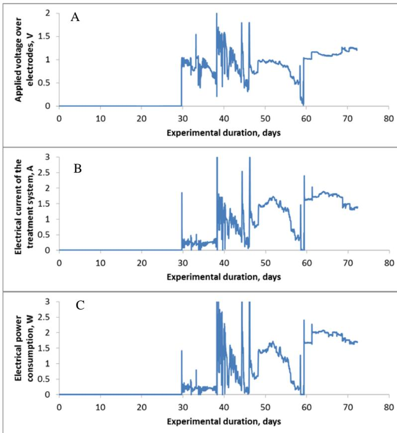
Figure 33. The applied voltage (A), monitored electrical current (B), and power consumption (C) in the electrode-assisted septic tank.
