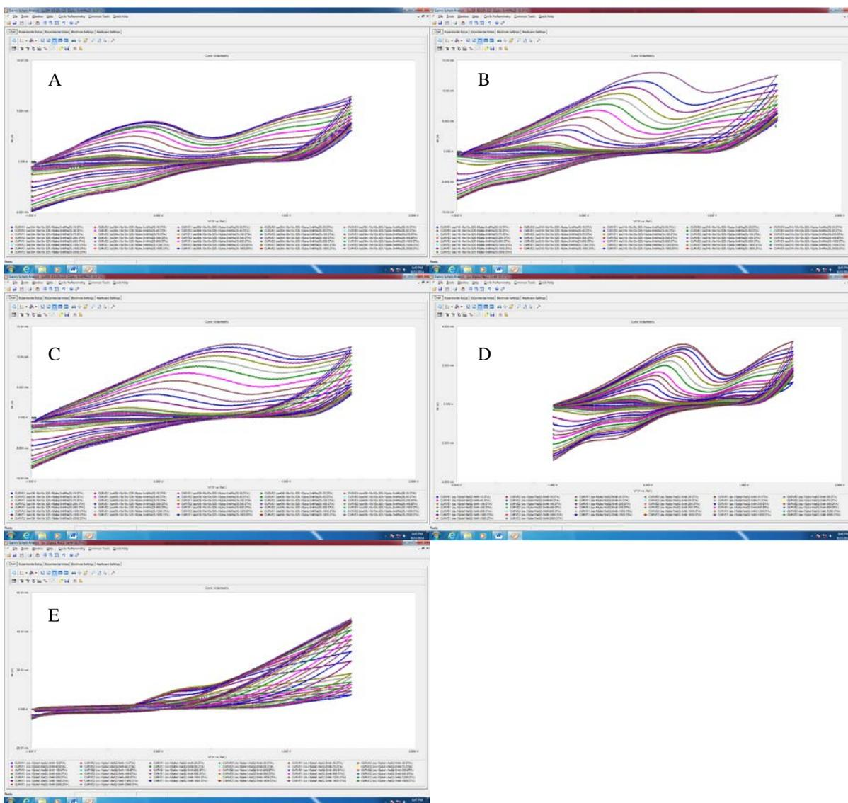
Figure 7. Cyclic voltammograms in phosphate buffer solution with Na<sub>2</sub>S (5 mM): A, SS 304 10; B, SS 316 10; C, SS 430 10; D, SS 304 4; and E, carbon cloth.
