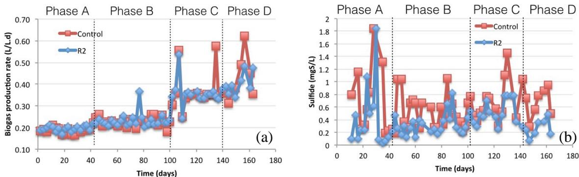
**Figure 22.** Biogas production rate (liters of biogas per liter of reactor per day) in both reactors, 'Control' reactor and CSTR-MEC reactor (R2). Sulfide concentration in the effluents in both reactors, 'Control' reactor and CSTR-MEC reactor (R2).
