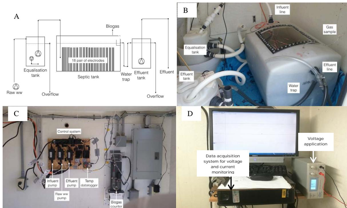
Figure 32. The process diagram (A), photo of septic tank (B), pump controlling system (C), and voltage application and monitoring system (D).
