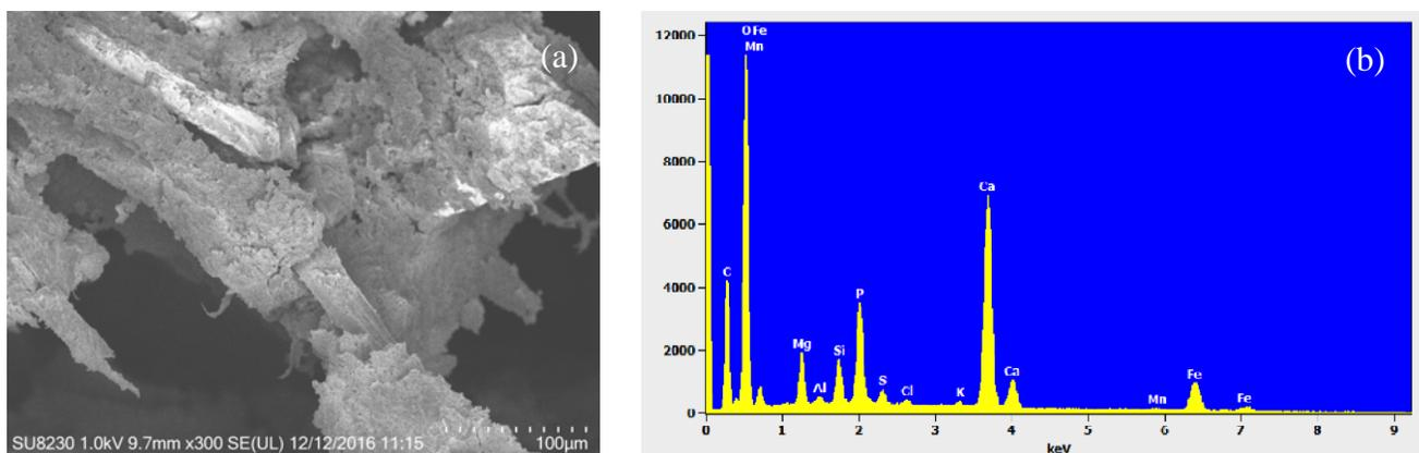
Figure 26. (a) SEM image of crystals on cathode surface; (b) Elemental surface analysis by EDS.
