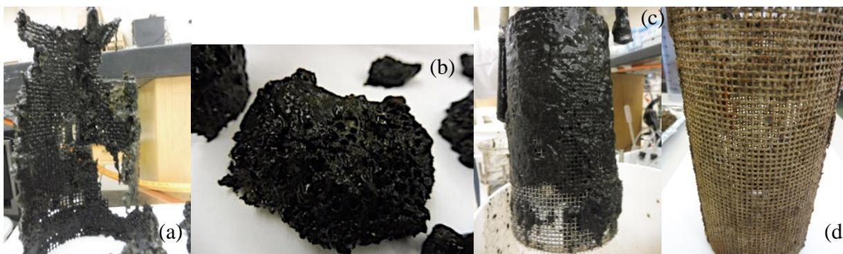
**Figure 23.** Visual observation of the electrodes after operating the reactors for about 160 days. (a) Anode in the CSTR-MEC reactor; (b) Anodic production of iron precipitates in the CSTR-MEC reactor; (c) Cathode in the Control reactor; (d) Cathode in the CSTR-MEC reactor
