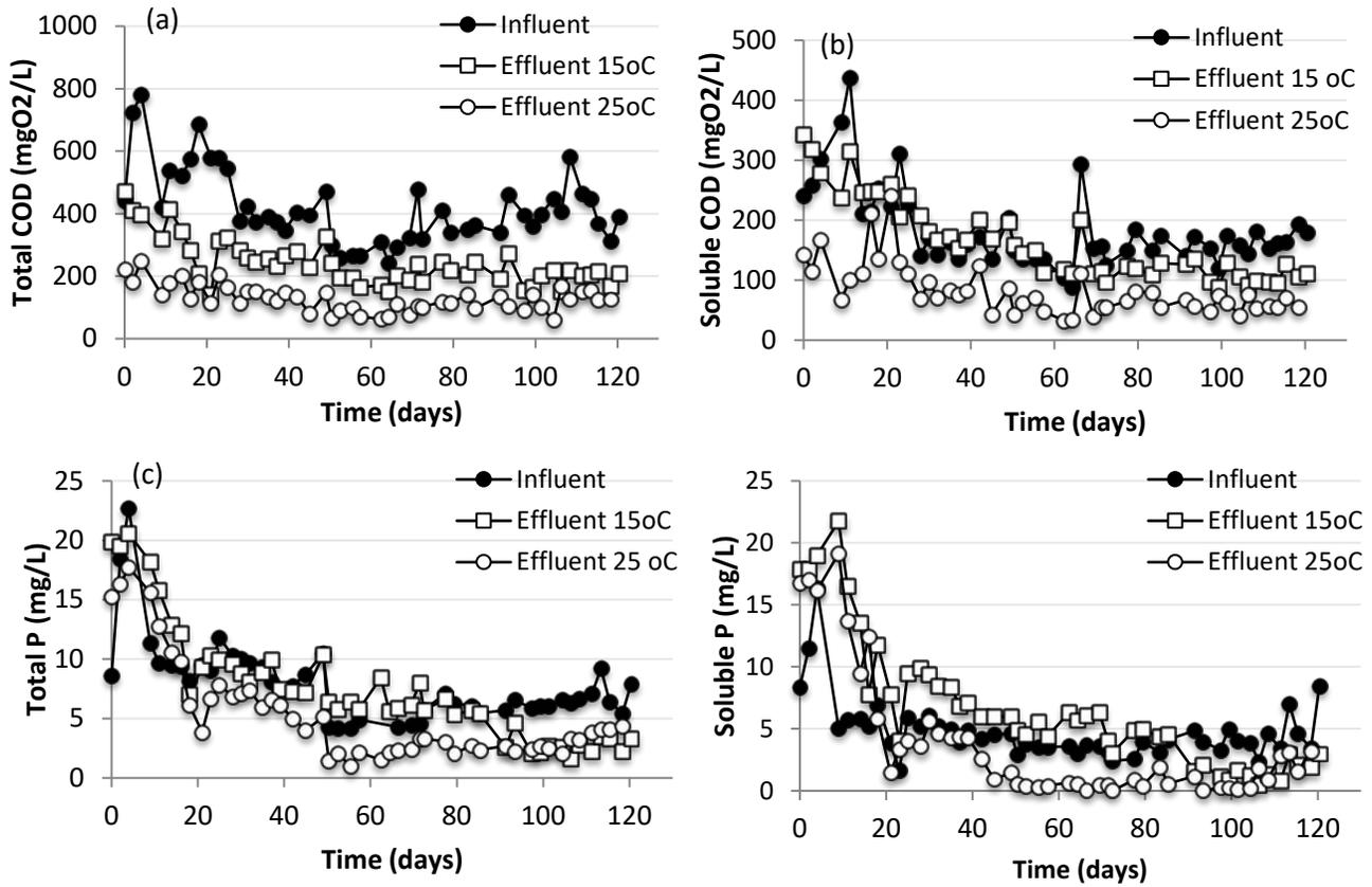
**Figure 30.** Evolution of the influent and effluent concentrations in the 20-liter lab-scale prototype reactors operated at 15 °C and 25 °C; (a) total chemical oxygen demand; total COD (b) soluble chemical oxygen demand; Soluble COD; (c) total phosphorous, total P and (d) soluble phosphorous, soluble P.
