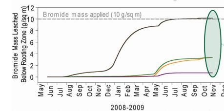
**Figure 6.** Cumulative bromide mass leached below the rooting zone (1.6 m below land surface).
