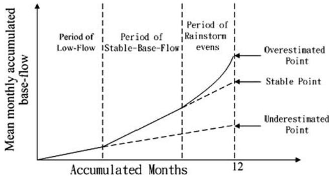
Fig. 2 The diagram of the stable-base-flow analysis
