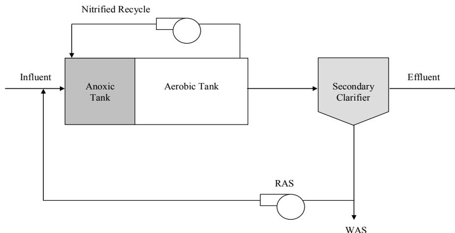
**Figure 1.** Taken from Kang et al. (2008). WAS is waste activated sludge. RAS is recycle activated sludge.
