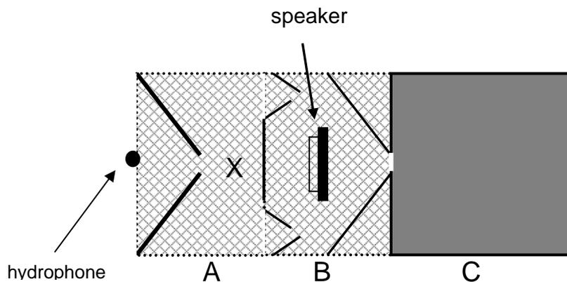
Figure 2. Round goby bioacoustic trap. The schematic displays a dorsal view of the trap. The first two sections (A and B) are composed of fine wire netting from modified minnow traps. The terminal section C is opaque. One way funnel entrances/exits (solid lines) lead into each section
