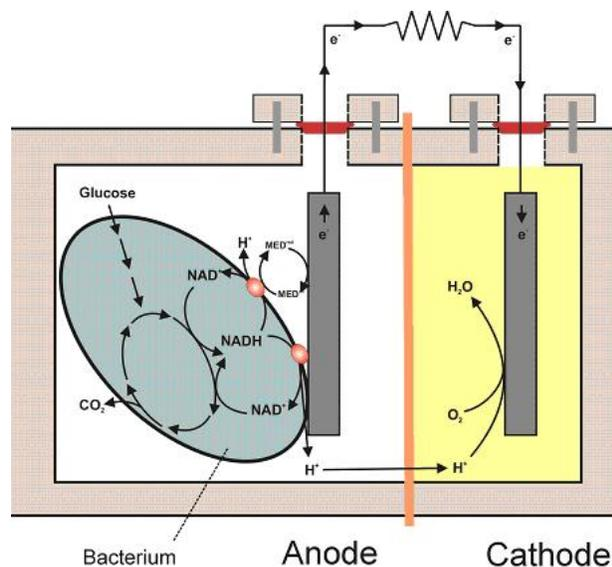
**Fig. 6.** Schematic of a microbial fuel cell. (microbialfuelcell.org)
