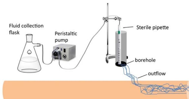
**Fig. 5.** Diagram of borehole water collection setup. A sterile pipette is suspended in the borehole and held in place by a clamp stand. Attached tygon tubing runs through a peristaltic pump set at half the outflow rate (0.5mL). The water is collected in a 2 liter Erlenmeyer flask that is collected and sterile filtered daily. Water would be collected for 2-3 days.
