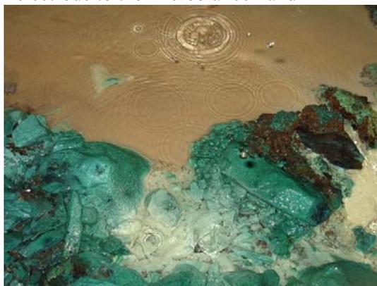
**Fig. 9.** Copper precipitation on level 10 of the Soudan Iron Mine.
