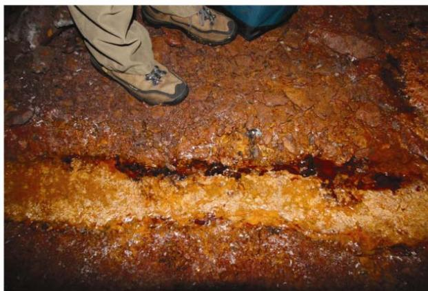
**Fig. 10.** Iron oxide ‘foam’ precipitated downstream from boreholes in the west tunnel of level 27.
