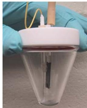
**Fig. 7.** Electrobioreactor for cathode experiments.
