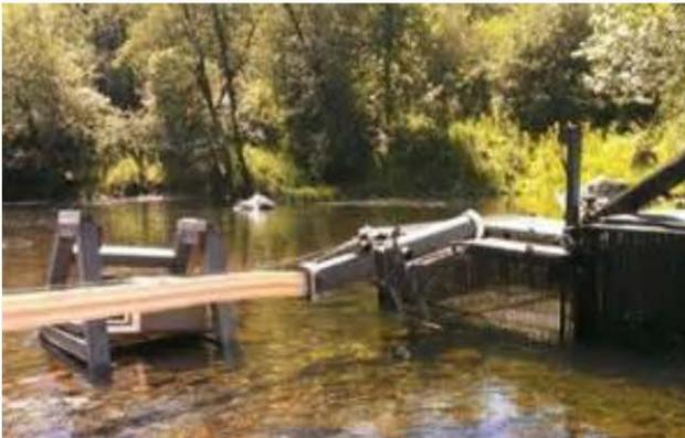
An existing technology developed to transport salmon over dams could be modified to remove migratory common carp from many barrier sites in MN
