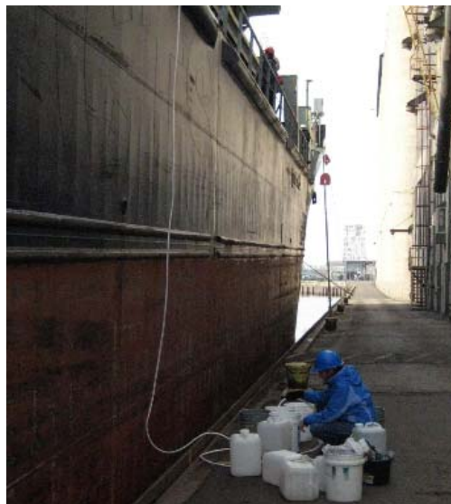
Fig. 1. Collection of a ballast water sample from a sounding tube of a commercial ship in the Duluth-Superior harbor.
